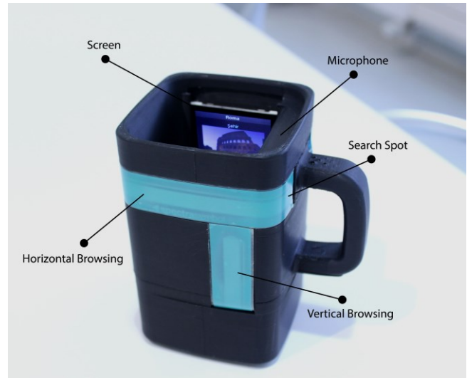
Figure 1. The Glance Mug prototype and system components
